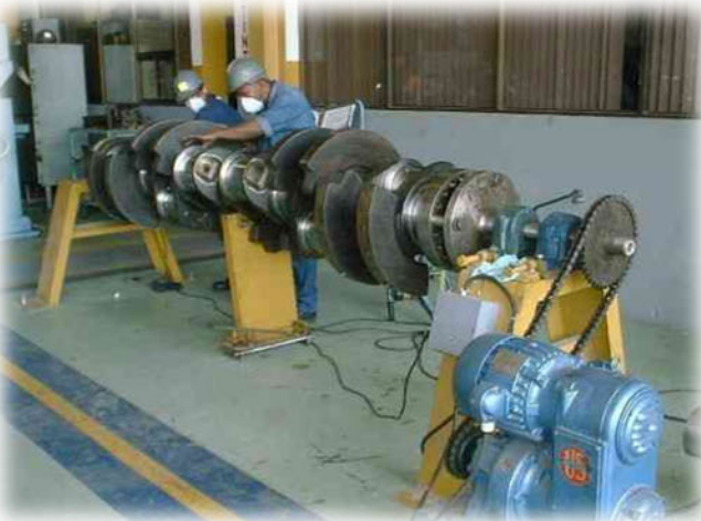
Measuring the crankshaft bearings for a Caterpillar® medium speed engine.
