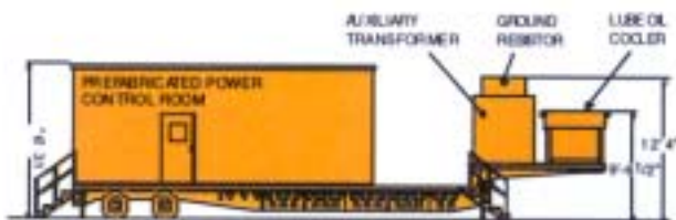
Power Control Module
